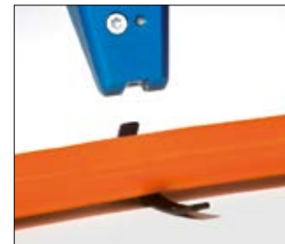
... release the push rod and remove the tool, the tie is cut.
