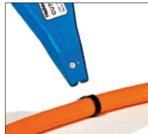
Bring the tool perpendicular on the tie...
