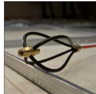
The whisk allows the rod to glide over obstructions easily.
